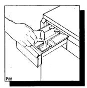
Pour the softener, if required, into the compartment marked **3**; do not exceed the MAX level.
